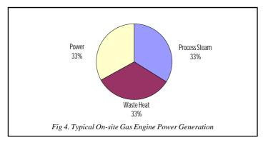
Figure 4 shows similar figures for a diesel or gas engine operation where it will be noted that nearly 35% of the fuel input can be converted to electricity with 67% waste heat, of which some 35% can be reclaimed for process steam.
