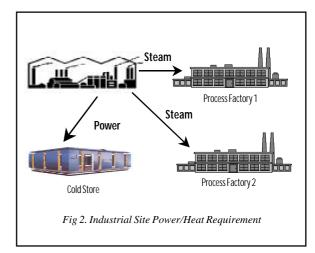
To better understand the concept, figure 2 shows an industrial site with the cold storage complex surrounded on two sides by process factories which would normally have their own separate boiler plant producing steam. A total energy solution would be to generate power on the site as shown, passing the power to the cold store operator who would then pass the waste heat (normally despatched to atmosphere) to the two respective factories.
