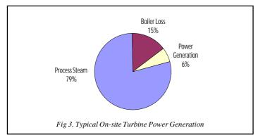
Figure 3 demonstrates a typical industrial low cost steam turbine performance showing energy conversion into electricity and process steam. The 6% power generation may appear small but this power is generated at nearly 100% efficiency rather than buying from a power station with an efficiency of 30%-35% to which transmission loss must be added, making the power station achieve a final energy conversion efficiency of no more than 25%.
